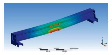
All Intermac products are designed with a CAD program for solid modelling that simulates the dynamic stress generated during the machining operations and highlights any areas that need to be stiffened in order to ensure long-lasting reliability for the machine.
