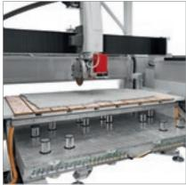
The wooden work table enters into the working area above the aluminium table, where the suction cups are already in place.
