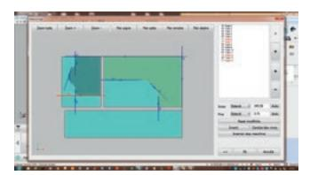
Optimise cutting operations on individual pieces within the nesting system by programming the order of cuts and the movement of pieces using the manipulator between one cut and the next.
