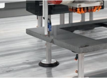
The variable Z thickness tracer (optional) maintains constant machining quality, even on pieces of irregular thickness. Also suitable inclined disc-cutting processes.
