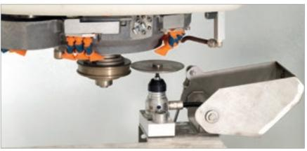
The mechanical pre-setter (optional) checks the degree of wear on the diamond tools (the frequency of these checks is set by the machine operator), and automatically updates the tool parameters in the machine control unit, thereby guaranteeing consistent machining results over time.
