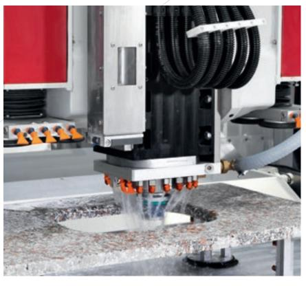
Spindle absorption is constantly measured by the NC, and the pressure exerted by the tool on the piece is then proportionally adjusted to guarantee the best possible finish quality.
