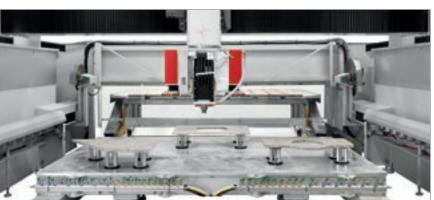
The pieces to be finished are placed on the aluminium table, ready to be processed.
