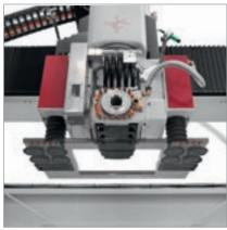
The semi-finished pieces are collected by the suction cup system on the head, and positioned on the aluminium table suction cups.
