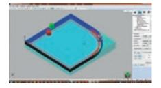
EasyCut: simplified interface for programming 3-axis disc machining operations.
