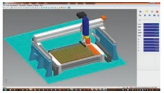
**Simulation on the virtual machine**: users can simulate the machine's entire working cycle, checking the movements of the head, the bench and the manipulator:
